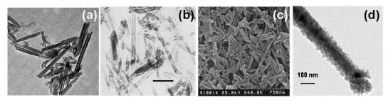
TEM images of halloysite nanotubes dispersed in water (a-b), SEM image of layer-by-layer nanocoating with halloysite multilayer (c), and halloysite nanotube coated with polyelectrolyte + 7 nm diameter silica
